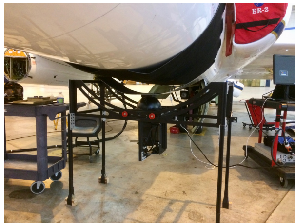
Figure 5. Linear integrating sphere on swinging track below the mounted AVIRIS-NG instrument in the flight hanger.
