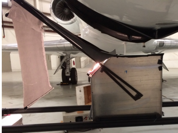
Figure 3. Apophotic box deployment for hanger calibration. The interior is lined with 2% black polishing cloth. On the top face of the box, there is an aperture enabling a view of the standard panel inside. A frame similar to arrangement on left controls lamp and panel geometry. Note curtain preventing reflected lamp light from illuminating the panel inside the box. For this (less portable) methodology, no background measurement is necessary.
