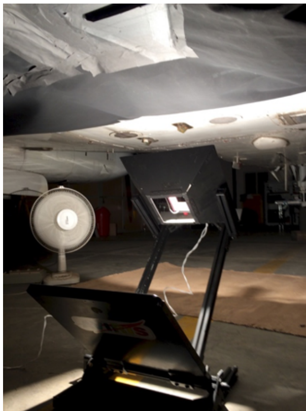
Figure 4. Lamp-and-panel frame with shutter deployment for hanger calibration. Shutter is deployed with lamp on. Data is then acquired for measurement of background illumination. Note entrance slit aperture of AVIRIS-NG at in aircraft belly at top of photo. This particular hangar cal was performed in the sub-tropics. The fan is to keep insects off of the lamp.
